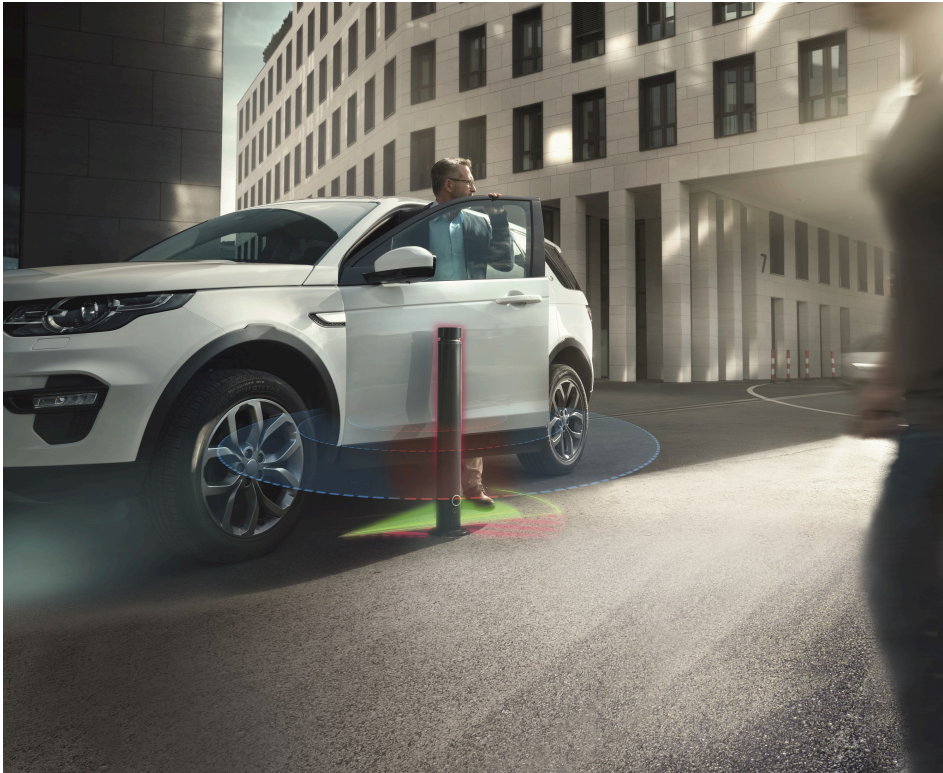
Radar sensors prevent collisions with the vehicle door. (Source: Brose)
