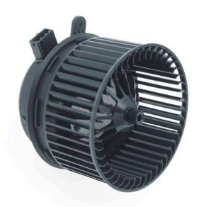
The use of a brushless motor with rare earth magnets reduces the weight of Brose's HVAC blower by some 700 grams compared to brushed variants. In addition, the overall length of these drives can be reduced by around 40 mm.
