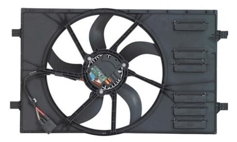
Brushless cooling fan module: With its new generation of brushless cooling fan modules, which will go into series production at the beginning of 2012, Brose will demonstrate an effective solution for engine cooling at this year's IAA: The overall length has been reduced by approx. 15 millimeters and the weight by some 700 grams.
