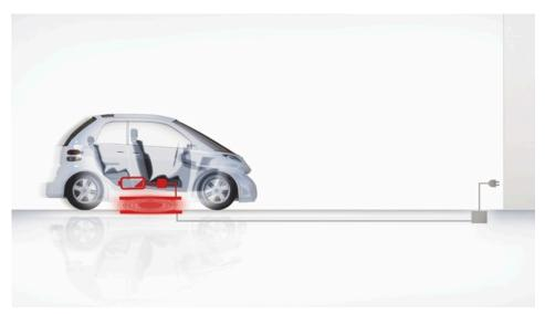
The principle of induction entails power being transmitted via an air gap of up to 20 cm. The coil which generates the magnetic field is embedded in the parking area. The counterpart to this is the receiver in the underbody of the vehicle.
