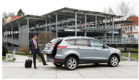
A simple foot movement below the bumper is all it takes to automatically open and close the liftgate. If desired, this feature can be connected to the cargo area cover, thus providing access to the cargo area as the liftgate opens. In addition, the opening angle of the liftgate can be individually programmed to fit the respective garage height.
