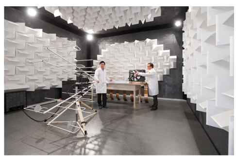
In its accredited test center in Würzburg, Brose test engineers check the electromagnetic compatibility (EMC) of up to 100 products of its door systems, seat systems and drives business divisions each year. The test results are incorporated early on in the product development and design.
