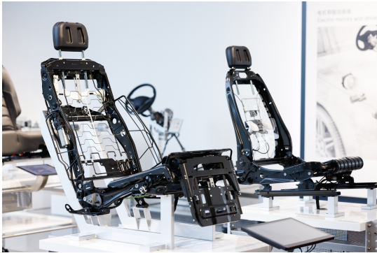
Brose electrically adjustable seat frame
