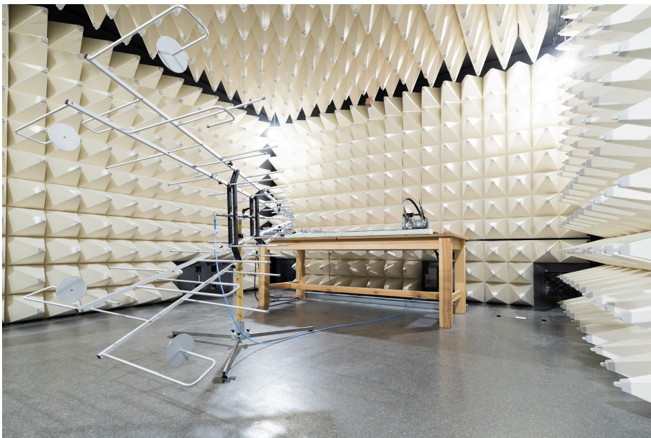
Following the expansion of the test center in Würzburg, Brose has four absorber chambers at its disposal.
