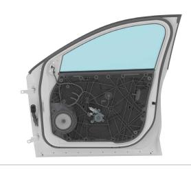
Structure modules made of organo sheet stand for cost-effective weight savings in the side door.
