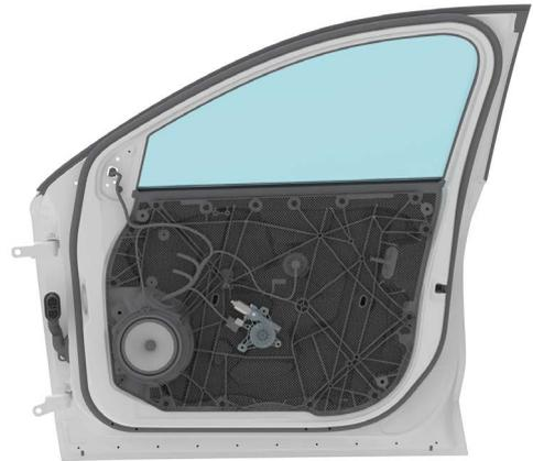
Structure modules made of organo sheet stand for cost-effective weight savings in the side door.
