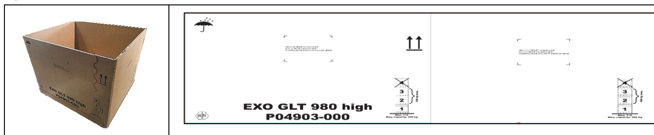
Illustration 37 - Placing of markings on GLT
