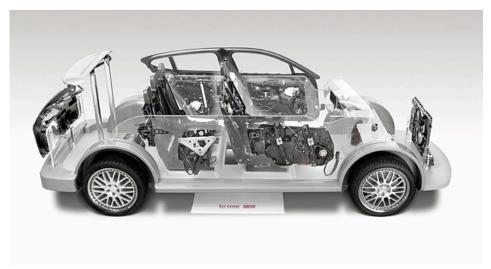
Brose's product portfolio spans from cooling fans to electric motors for vehicles and power liftgates.
