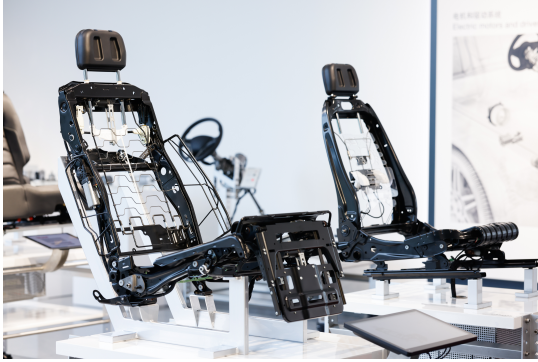
Brose electrically adjustable seat frame
