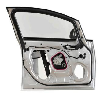
Brose will present a window regulator made of long glass-fiber reinforced polypropylene with integrated guide rails and wet/dry side separation for the first time at the IAA 2011. A foam-filled seal on the base plate of the window regulator system allows the positioning of motor, electronics and wiring on the dry side.
