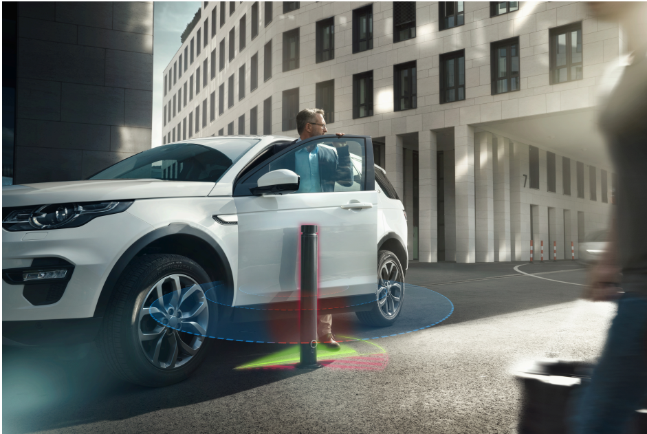
Brose side door drive with radar collision protection. The automotive supplier's mechatronic systems make vehicle access safer and more comfortable and convenient than ever before.
