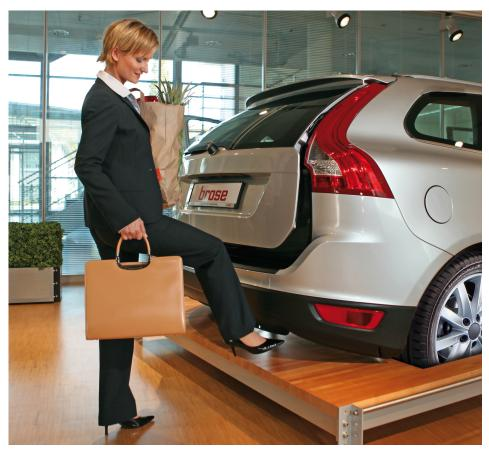
The capacitive liftgate switch makes loading and unloading of vehicles even more convenient. In conjunction with the keyless entry function, a simple foot movement is all that's needed for the lid to open by itself.
