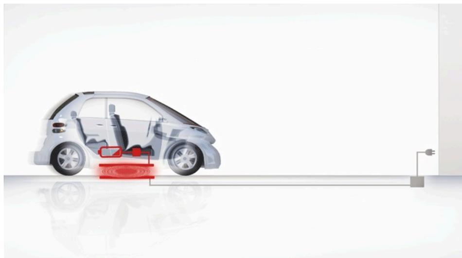
The principle of induction entails power being transmitted via an air gap of up to 20 cm. The coil which generates the magnetic field is embedded in the parking area. The counterpart to this is the receiver in the underbody of the vehicle.
