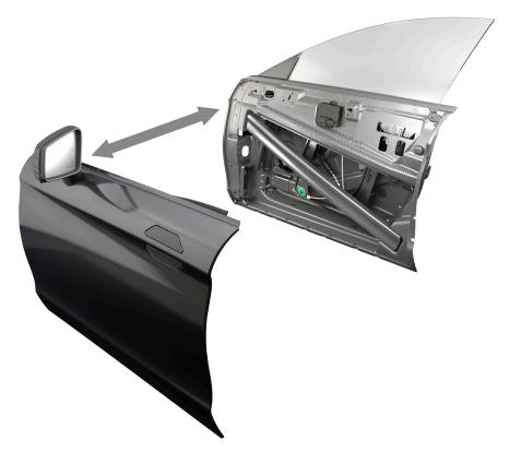
Brose's CFRP door structure delivers maximum functional integration, thereby reducing the number of parts and hence costs significantly. OEMs only need to mount and screw on the outer door panel, which considerably reduces assembly time.
